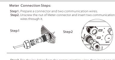
Step3. Trip the insulation from the communication wires, then insert one side of wires into pin1 and pin 2 holes of the 8 pin positive terminal which can be found in accessories package. And then screw them tightly.
